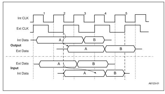
Figure 16-17. Processor 2/3 Bus Internal/External Data Movement
